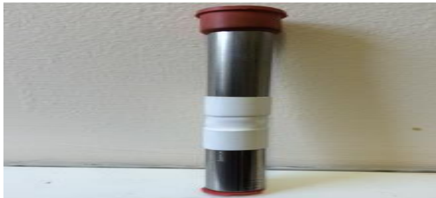
Figure 3.A metal tube for the accumulation and collection of ethylene gas
